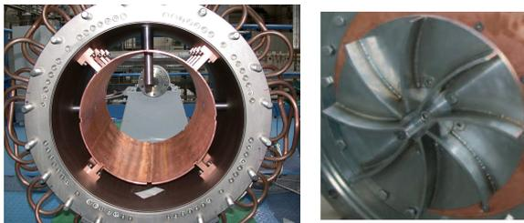
Figure 1: *VKS2 flow vessel and driving impellers*
