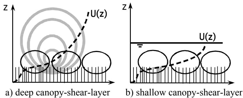
**Figure 1.** a) In deep canopy-shear-layers K-H vortices (black) interact with larger-scale boundary-layer turbulence (grey). B) In shallow canopy-shear-layers K-H vortices may dominate through the flow domain.
