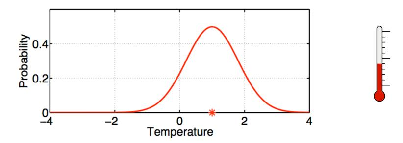
Instrument builder says thermometer is unbiased with +/- 0.8C gaussian error.
