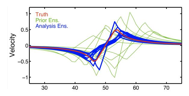
Transform state to position and wind relative to center. Assimilate observation of wind and position. Transform back. Invertible transformation of state before assimilation
