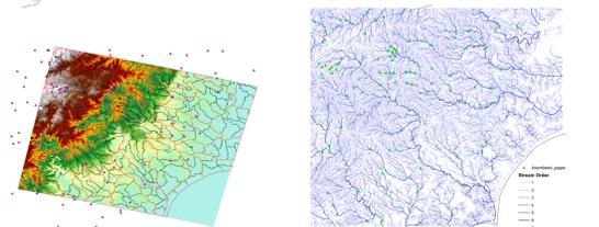
**Figure 8:** Left: The test domain 'Matthew' for WRF-Hydro and DART. The domain is approximately 100,000 km<sup>2</sup>. The triangles are at stream gage locations. The LSM runs at ≈ 1 km resolution. Right: A depiction of the Stream Order.
