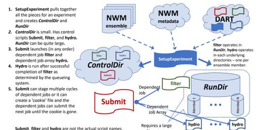
**Figure 10:** Schematic of the workflow of WRF-Hydro and DART. Separate jobs perform the assimilation and a Job Array is used to run the ensemble of WRF-Hydro instances. Each job can be tuned for an optimal configuration. Since each job runs for a very short time, the jobs may backfill. The queuing system takes care of the job dependencies and automatically resubmits the next job in the series.
