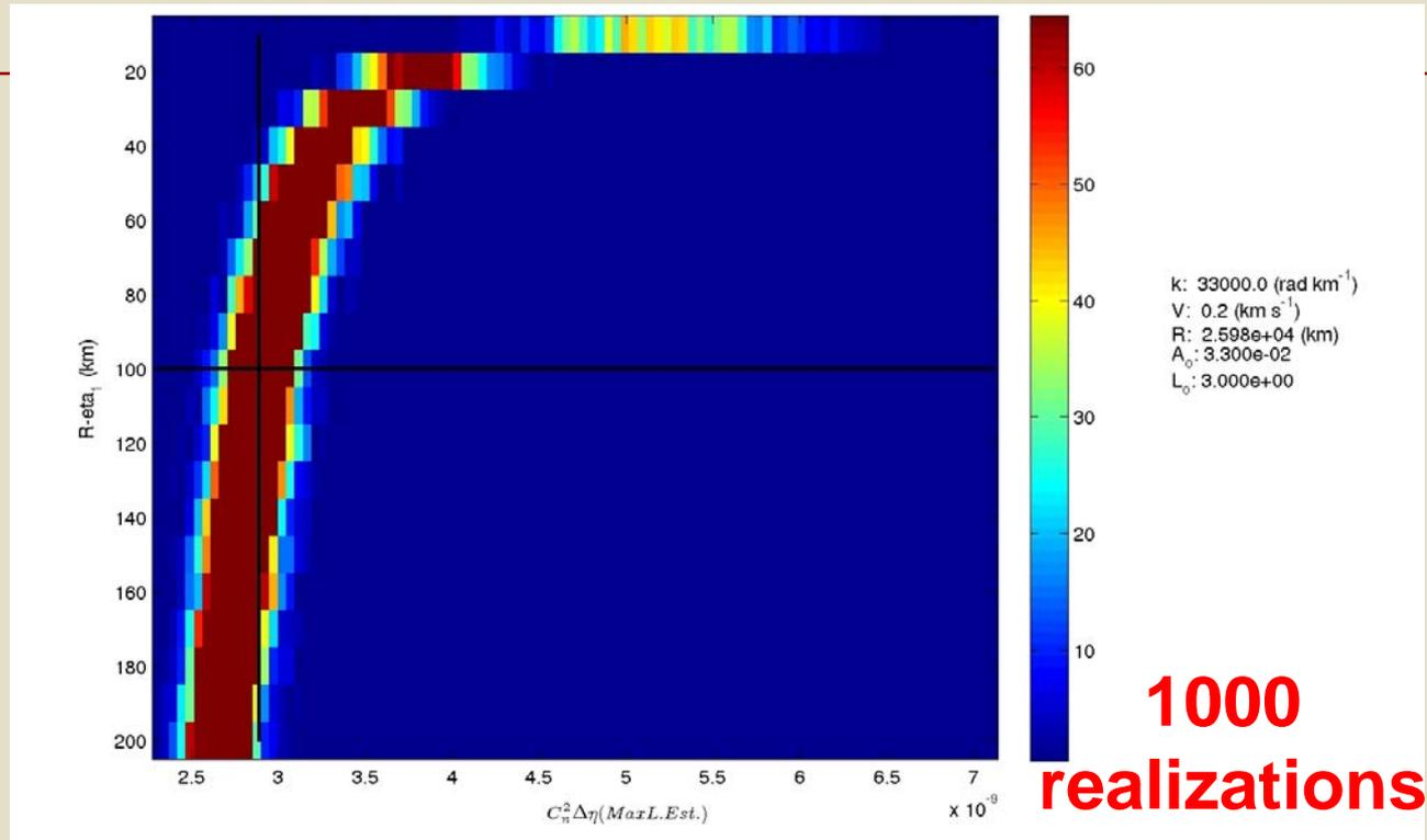
ML estimation of intensity with fixed  $L_0 = 3 \text{ km}$  while varying  $R - \eta_1$ .
