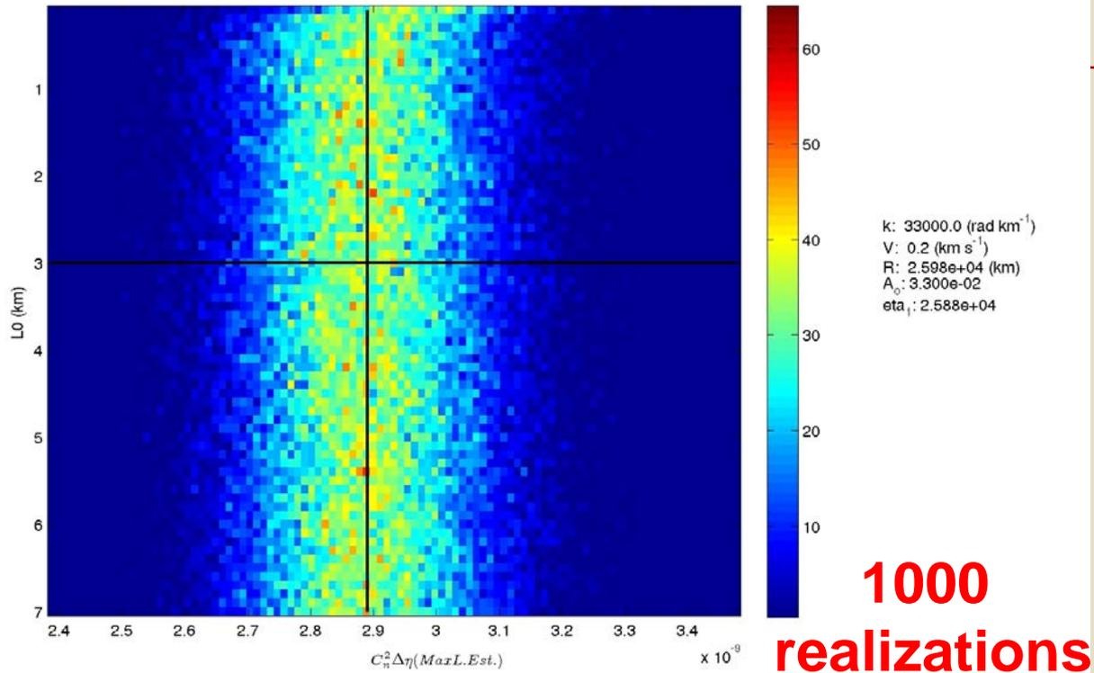
Maximum Likelihood (ML) estimation of intensity with fixed  $R - \eta_1 = 100 \text{ km}$  while varying  $L_0$ . Horizontal and vertical lines are simulated (i.e., “true”) values.
