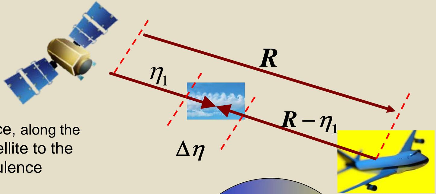
$\eta_1$  is the distance, along the LOS, from the satellite to the center of the turbulence patch.
