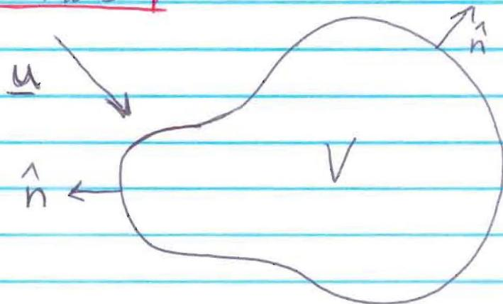
$$\frac{d}{dt} \int_V \rho dV = \frac{\text{mass in - mass out}}{\text{unit time}} = \int_A \rho (-\underline{u} \cdot \hat{n}) dA$$
