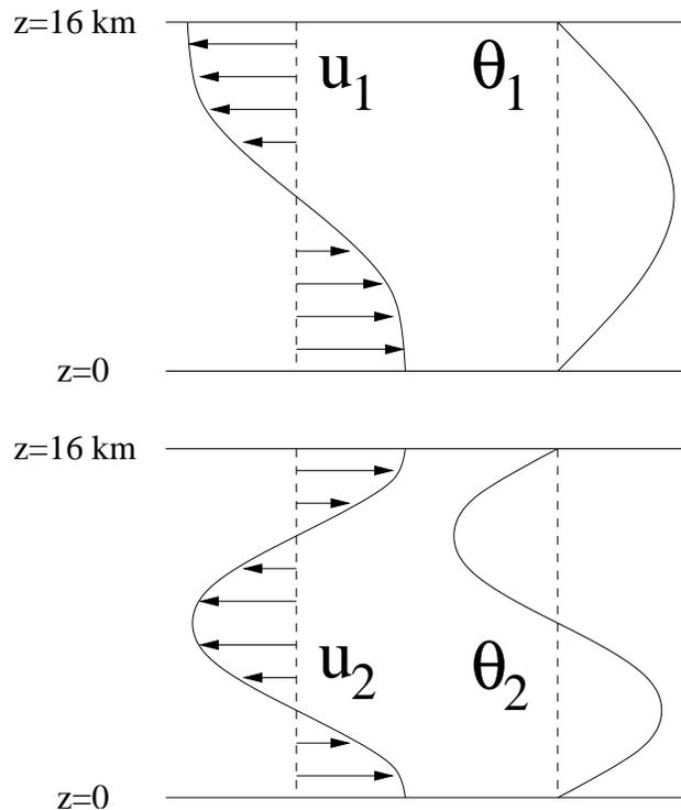
$$\begin{cases} \frac{\partial u_1}{\partial t} - \frac{\partial \theta_1}{\partial x} = -\frac{1}{\tau_u} u_1 \\ \frac{\partial \theta_1}{\partial t} - \frac{\partial u_1}{\partial x} = H_d - R_1 \end{cases}$$
