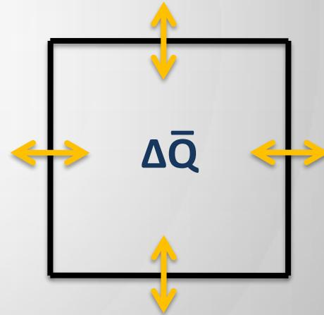
$$\bar{Q}^{n+1} = \bar{Q}^n - \frac{\Delta t}{V_{\Omega}} \sum_i \Gamma_i F_{avg,i}^{\perp}$$
