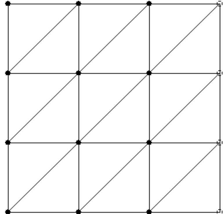
**Coarse Grid Solve:** Poisson problem using linear finite elements on entire spectral element mesh,  $A_0$  (GLOBAL).
