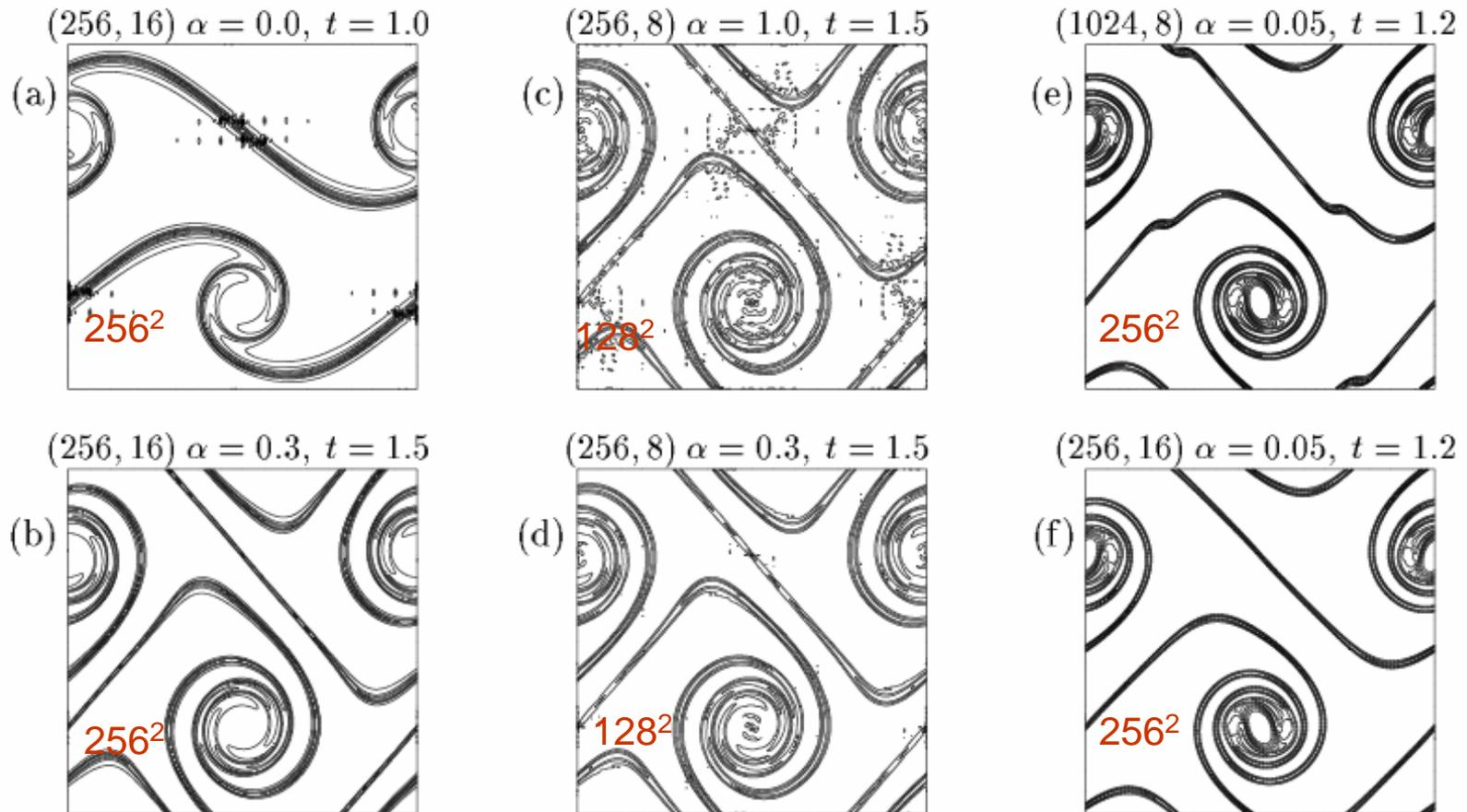
Figure 1: Vorticity for different  $(K, N)$  pairings: (a-d)  $\rho = 30$ ,  $Re = 10^5$ , contours from -70 to 70 by 140/15; (e-f)  $\rho = 100$ ,  $Re = 40,000$ , contours from -36 to 36 by 72/13. (cf. Fig. 3c in [4]).
