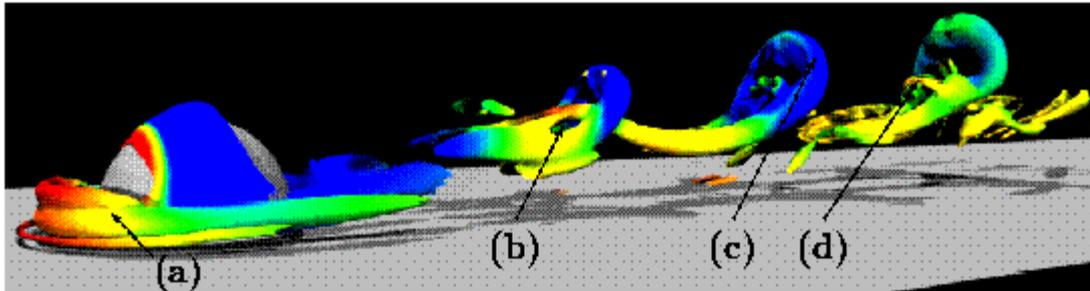
Figure 1: Principal vortex structures identified by  $\lambda_2 = -1$  isosurfaces at  $Re_* = 760$ : standing horseshoe vortex (a), interlaced tails (b), hairpin head (c), and bridge (d). Colors indicate pressure. ( $K=1021$ ,  $N = 15$ ).
